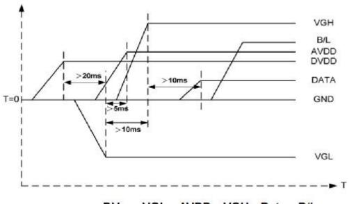
$DV_{DD} \rightarrow VGL \rightarrow AVDD \rightarrow VGH \rightarrow Data \rightarrow B/L$
