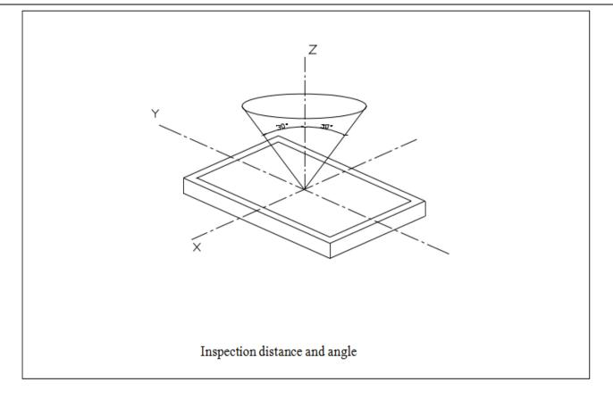
Inspection should be performed within angle $\varphi(\varphi$  is usually 30°) from Z axis to each X and Y.Inspection distance in any direction within  $\varphi$  must be kept 30±5cm from the display surface.
