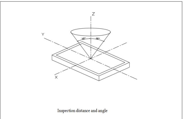
Inspection should be performed within angleφ(φis usually 30°) from Z axis to each X and Y.Inspection distance in any direction within omust be kept 30±5cm from the display surface.
